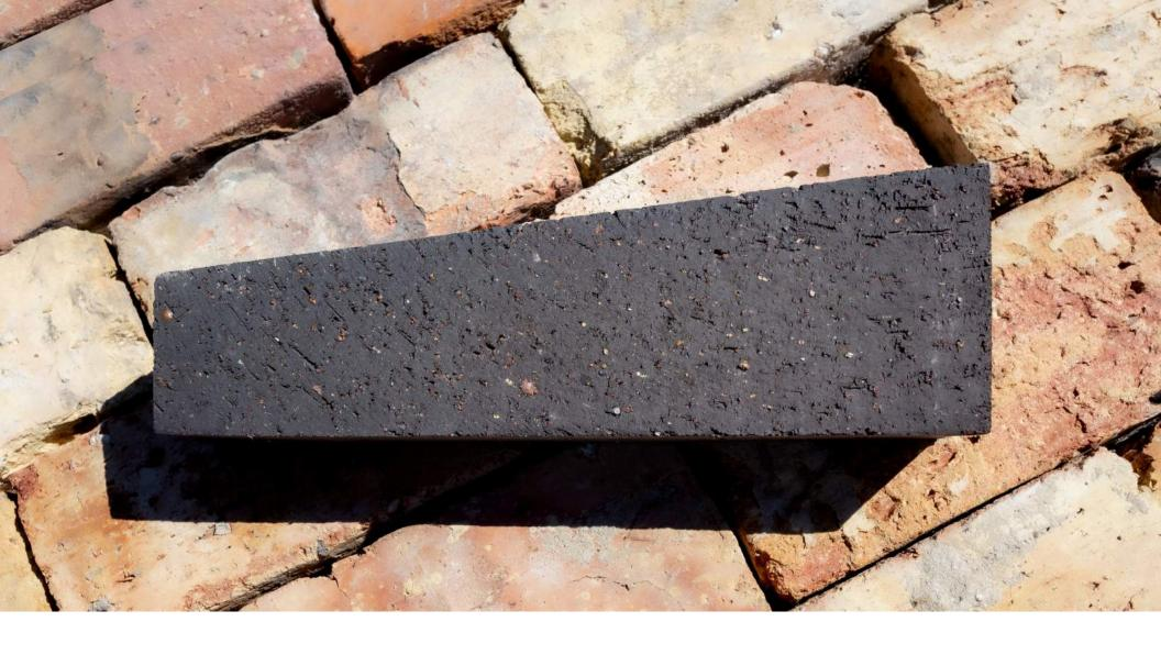
The flat back made the laying of each brick in line an easy task and the angled front created the angled effect at a consistency that would not have been possible with a rectangular brick.
