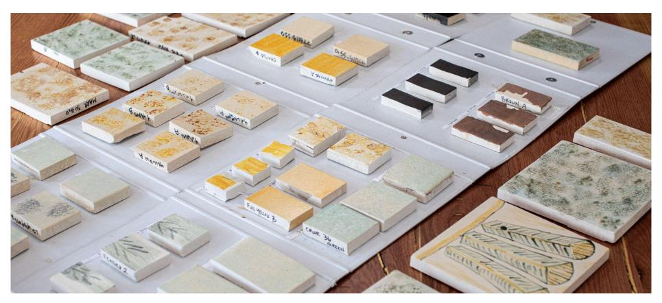
They tried applying the layers of glaze with brushes, with towels, with rollers, by spraying. "And you don't really know what you're going to get because the glaze is a totally different weapon when its fired," says Kafer.
